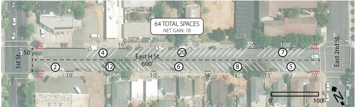
Figure 5: East H Street between 1st Street and East 2nd Street One lane eastbound with angle parking on both sides
